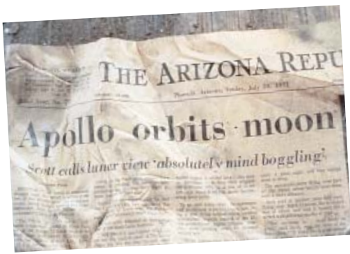
Figure 8 ► Biodegradable materials do not degrade quickly in modern landfills. This newspaper was put in a Tempe, Arizona landfill in 1971 and was removed in 1989.
