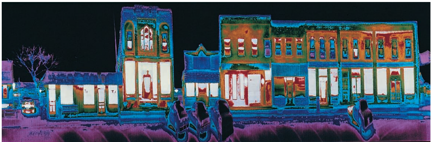
Figure 16-9 This thermogram , or infrared photo, shows heat losses (red, white, and orange) around the windows, doors, roofs, and foundations of houses and stores in Plymouth, Michigan (USA). Many homes and buildings in the United States and other countries are so full of leaks that their heat loss in cold weather and heat gain in hot weather are equivalent to what would be lost through a large, window-sized hole in a wall of the house. Question: How do you think the place where you live would compare to these buildings in terms of heat loss and the resulting waste of money spent on heating and cooling bills?
